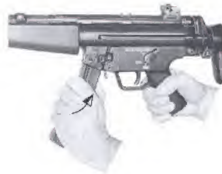
Fig. 24 Inserting the magazine
